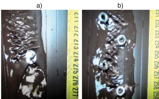
**Fig. 2. Zones of flow turbulization before and behind the obstructions in the form of inverted ball segment**
